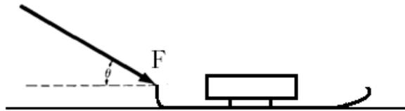
2. A boy pushes a 10 kg sled at a constant speed by applying a force of 75 N at  $30^\circ$  with respect to the horizontal. The sled is pushed over a distance of 15 m.
